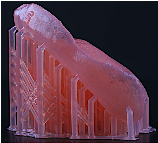
Figure 3: Image of a printed denture base before removal of the support structures. Notice the number “5”, which means this denture base was fabricated from impression number 5.
