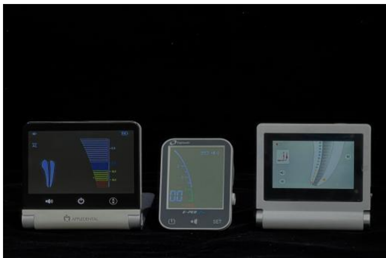
Figure 1: The three electronic apex locators assessed in this study are AppleDent AL (left), Eighteenth AL (center), and Coxo AL (right).
