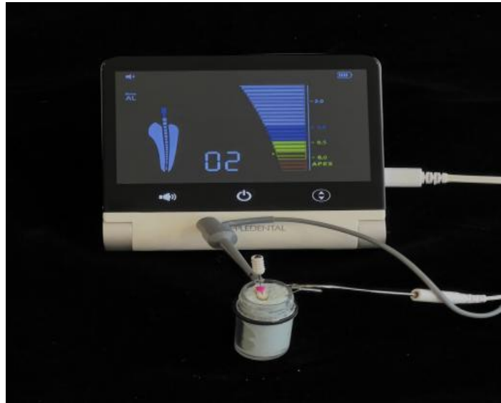
Figure 2: Experimental configuration illustrating the AppleDent electronic apex finder linked to a tooth encased in alginate for the purpose of ascertaining working length.
