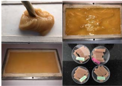
Figure 1: Silicon material in a customized metal mold.
