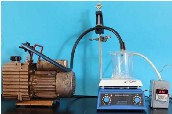
Figure 3: Bowl of the vacuum mixer connected to rotary pump and placed over magnetic hotplate stirrer to fasten the evaporation of the ethanol.
